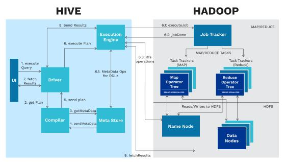
The diagram above shows how a typical query flows through Hive. The UI calls the Execution Engine through the Driver (step 1 in the diagram). The Driver creates a session handle for the query and sends the query to the Compiler to generate an execution plan (step 2).
